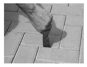
Figure 13. A simple test with a putty knife checks consolidation of the joint sand.
